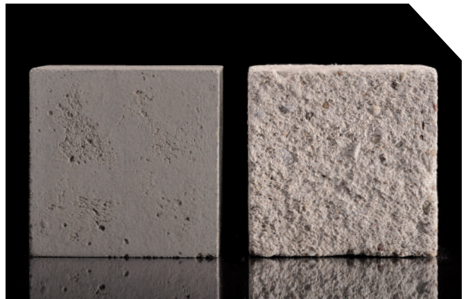
Figure 4: Istra 40 mortar (left side) and OPC mortar (right side) after 72h of corrosion in 10 % sulfuric acid
