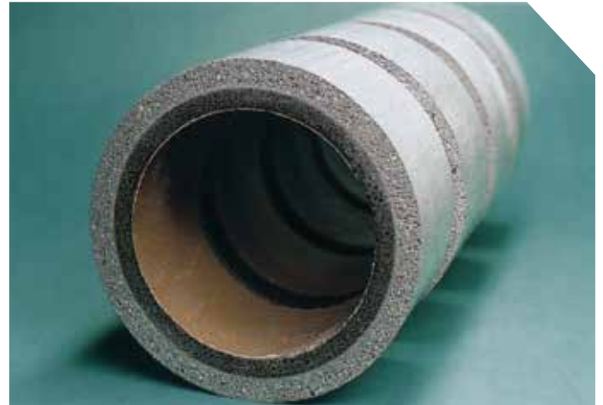
Figure 7: OPC concrete pipe with ISTRA 40 inliner
