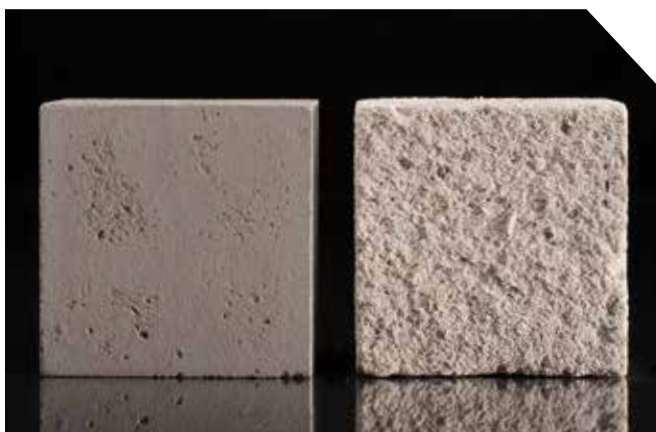
Figure 4: Istra 40 mortar (left side) and OPC mortar (right side) after 72h of corrosion in 10 % sulfuric acid
